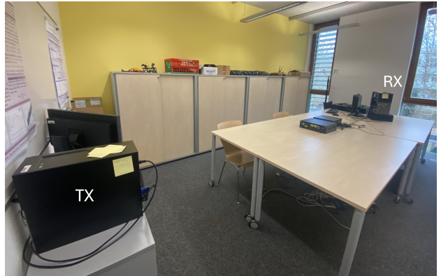
Fig. 1: Office room with experimental setup for Wi-Fi-based people detection and counting
