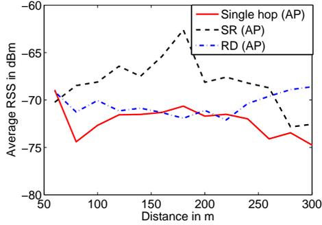
Fig. 4. Average RSS versus distance for single and two-hop setups.
