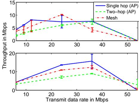
Fig. 5. Throughput for fixed rates for  $P_{TX} = 12$  dBm (upper) or 20 dBm (lower).
