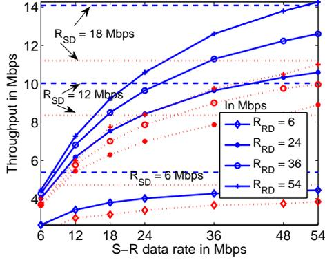
Fig. 2. Theoretical and measured (indoor) throughput over source-relay data rate ( $R_{SR}$ ) for single and two-hop 802.11a links. All rates are in Mbps.
