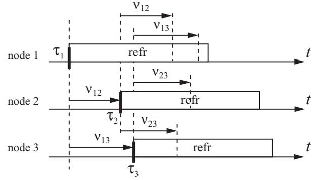
Fig. 3. Synchronization interactions for three nodes connected all-to-all.
