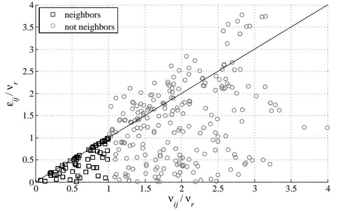
Fig. 5. Scatter plot of the achieved accuracy  $\epsilon_{ij}$  as a function of the propagation delay  $\nu_{ij}$  for a network of  $N=25$  with normalized connectivity  $\kappa/N=0.1$ .
