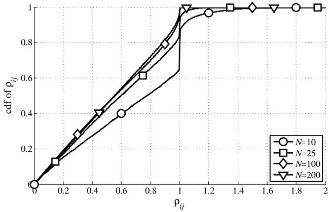
Fig. 7. Cdf of the normalized accuracy for networks of algebraic connectivity  $\kappa/N=0.1$ .
