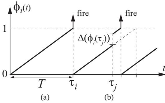
Fig. 1. (a) Uncoupled PCO phase function and (b) Phase increment upon reception of a pulse.
