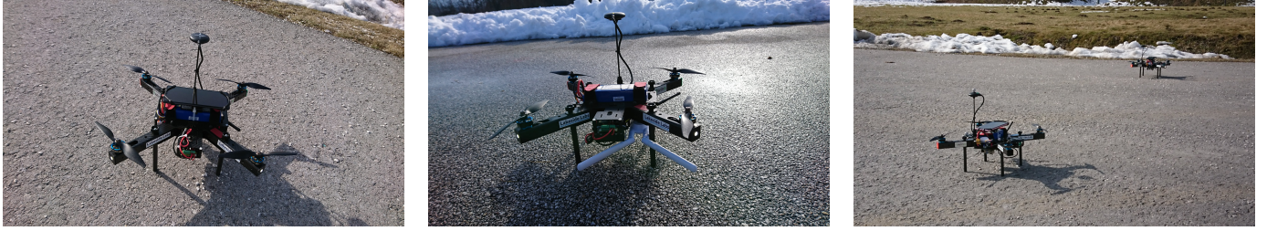
Fig. 2: Pictures taken during experiments. From left to right: (i) drone carrying a smartphone, (ii) drone carrying the Wi-Fi AP and (iii) both drones carrying a smartphone each.
